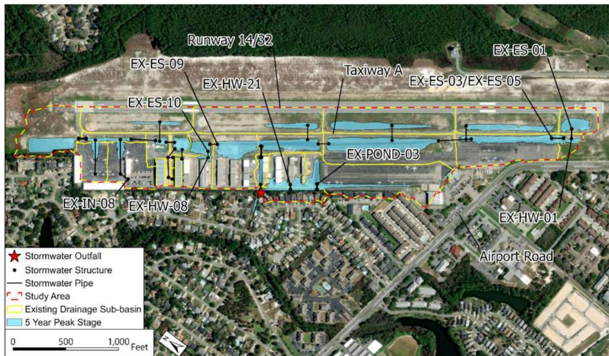
Figure 6-1: Existing Conditions – Existing Infrastructure 5-year, 24-hour Inundation Map
