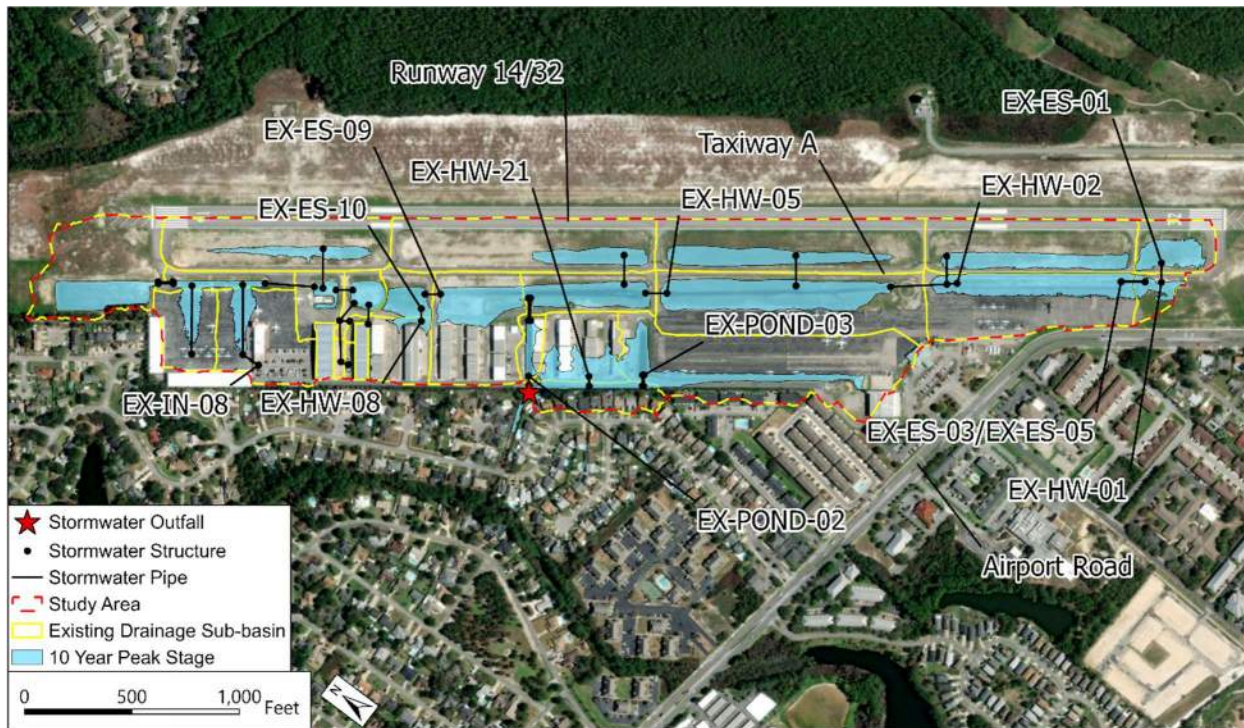
Figure 6-2: Existing Conditions – Existing Infrastructure 10-year, 24-hour Inundation Map
