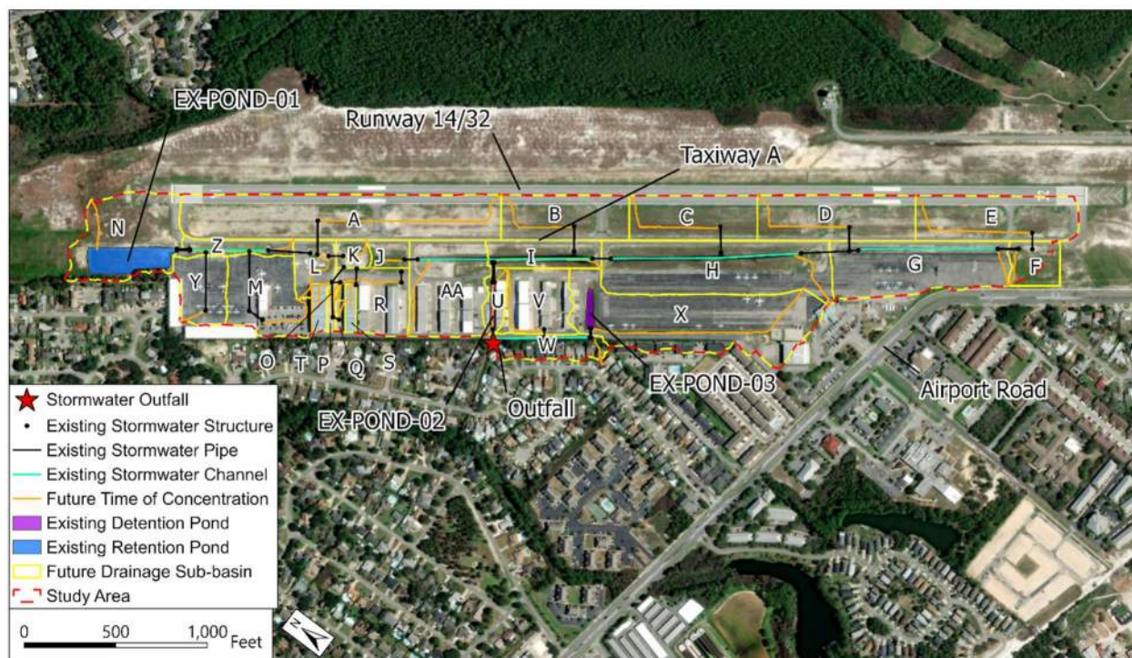
Figure 4-2: Future Hydrology and Existing Stormwater Infrastructure
