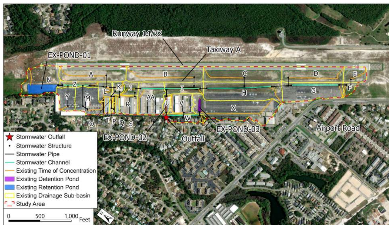
Figure 3-1: Existing Hydrology and Stormwater Infrastructure
