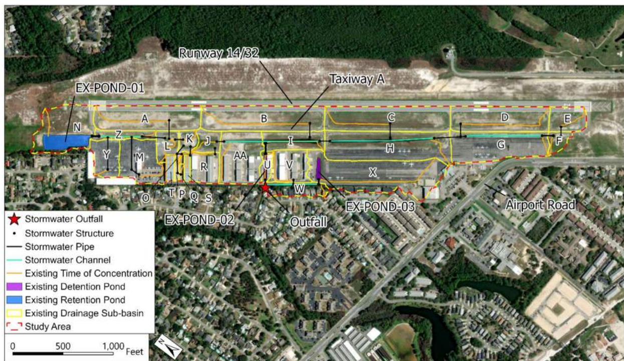
Figure ES-2: Existing Hydrology and Stormwater Infrastructure
